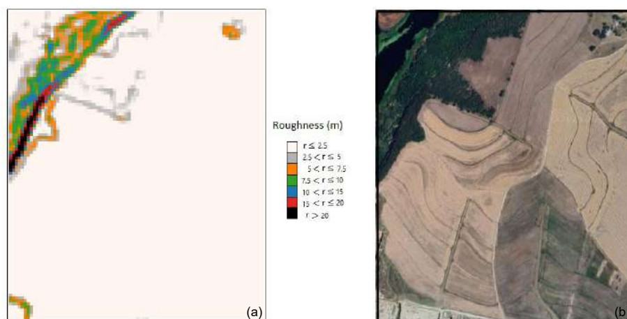
Figure 3. (a): Roughness image ( r ) obtained from GDAL plugins showing the maximum height differences between each pixel and the surrounding cells. (b): Satellite image obtained from Maxar Technologies Google Earth Pro on 2022/12/12.
